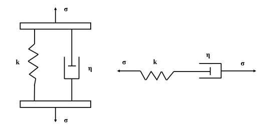
Figure 2.1 Voigt (Left) and Maxwell (Right) Rheological Models
