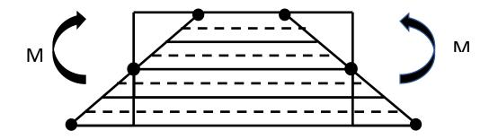
Figure 4.3 Through Thickness Shell Elements Bending in Abaqus
