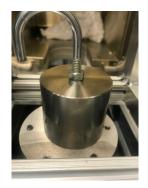
Figure 3.20 Counter Mass for Tape Springs' Structural Testing
