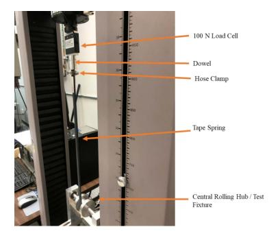
Figure 3.19 Tape Spring Boundary Conditions in Experimental Testing
