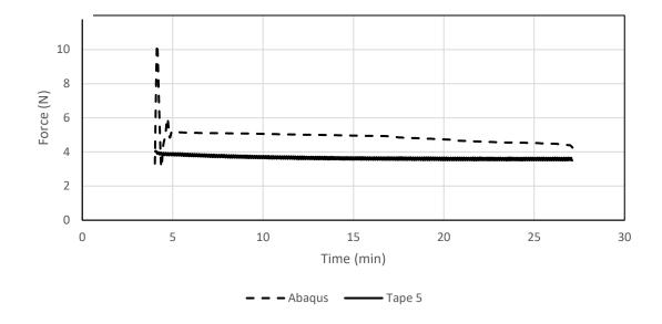
Figure 5.34 Comparison of Abaqus Predicted Results and Experimental Structural Test Results for Median ANP Tape Spring (Tape 5) for One Month Stowage
