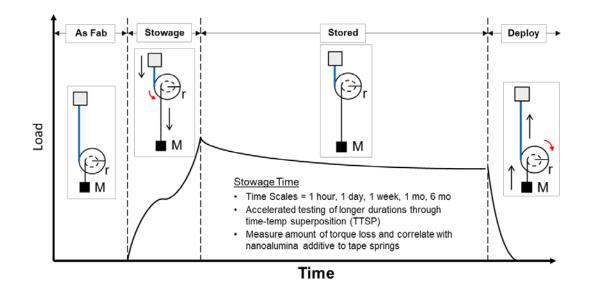
Figure 3.22 Tape Spring Structural Testing Load Profile
