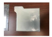
Figure 3.8 Neat Epoxy Sample #2
