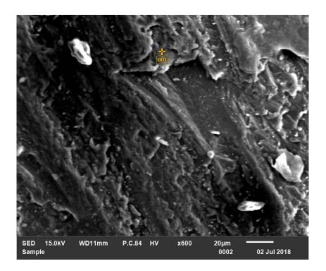
Figure 3.47 SEM Image of Analysis Point on ANP Epoxy
