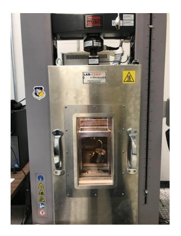
Figure 3.14 Lab-Temp Thermal Chamber
