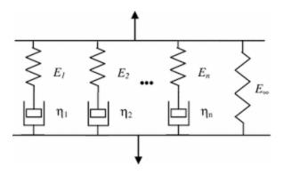
Figure 2.2 Generalized Maxwell Rheological Model
