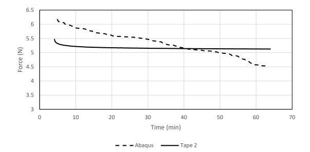
Figure 5.32 Comparison of Abaqus Predicted Results and Experimental Structural Test Results for Median ANP Tape Spring (Tape 2) for One Hour Stowage
