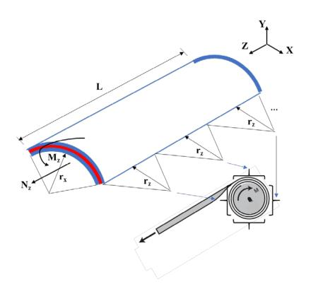
Figure 4.7 Tape Spring Load Geometry and Equal Sense Bending/Rolling
