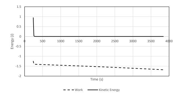
Figure 5.30 Energy Analysis for Step 3 of Abaqus Simulation of ANP Tape Springs with One Hour Stowage
