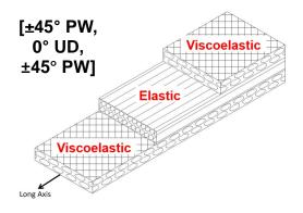
Figure 3.1 FlexLam Composite Laminate Layup
