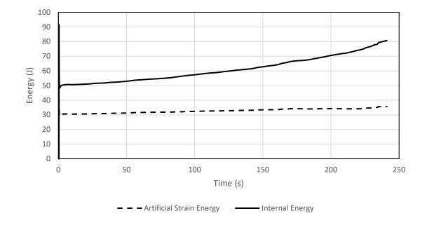
Figure 5.29 Energy Analysis for Steps 1 and 2 of Abaqus Simulation of ANP Tape Springs with One Hour Stowage
