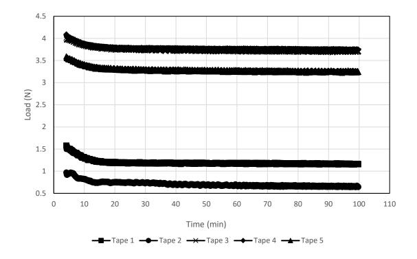
Figure 5.8 Control Tape Springs Six Months Stowage (via TTSP) Results Showing Loss in Deployment Force Over Time
