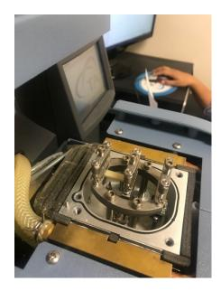
Figure 3.27 DMA Testing of ANP Coupons
