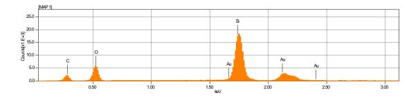
Figure 3.38 SEM/EDS Analysis of Control Tape Spring
