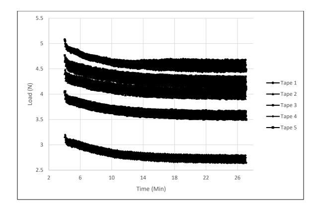
Figure 5.19 ANP Tape Springs One Month Stowage (via TTSP) Results Showing Loss in Tape Spring Deployment Force Over Time
