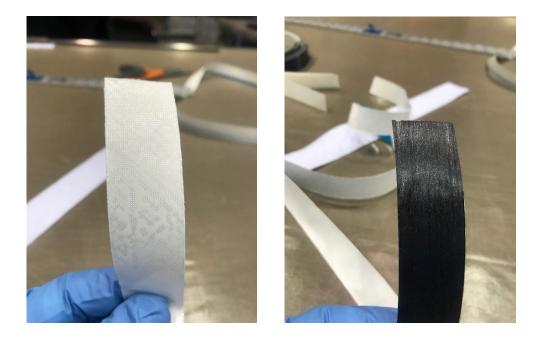
Figure 3.28 PW Prepreg and UD Prepreg
