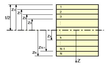
Figure 4.6 Geometry of N-Layered Composite Laminate
