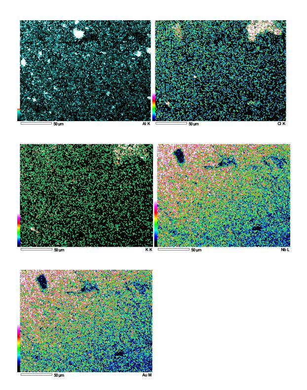
Figure 3.44 SEM/EDS of ANP Epoxy
