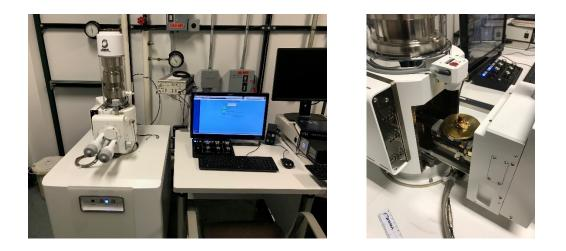
Figure 3.34 JEOL-JSM-IT100 SEM/EDS for ANP Dispersion Examination
