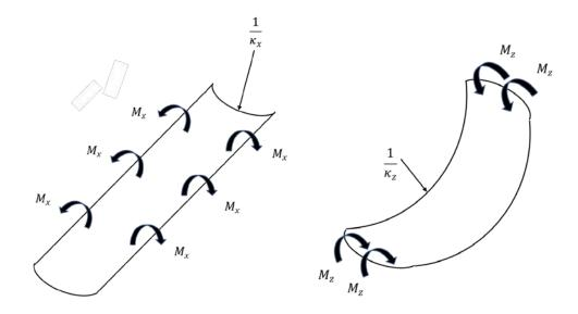
Figure 4.9 Bending Moments and Curvatures in Tape Spring
