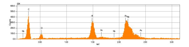
Figure 3.46 ANP Epoxy Elemental Composition (Box Analysis)
