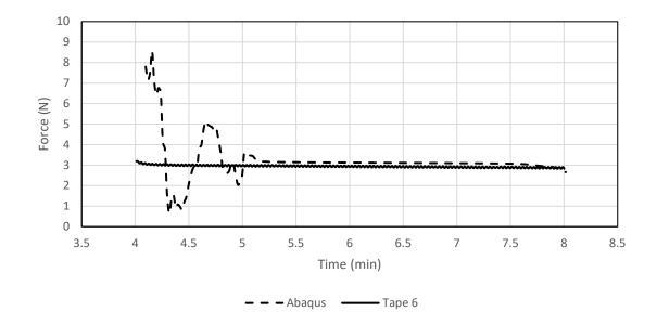
Figure 5.26 Comparison of Abaqus Predicted Results and Experimental Structural Test Results for Median Control Tape Spring (Tape 6) for One Week Stowage
