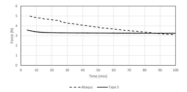
Figure 5.28 Comparison of Abaqus Predicted Results and Experimental Structural Test Results for Median Control Tape Spring (Tape 5) for Six Months Stowage
