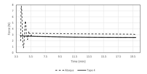
Figure 5.27 Comparison of Abaqus Predicted Results and Experimental Structural Test Results for Median Control Tape Spring (Tape 4) for One Month Stowage
