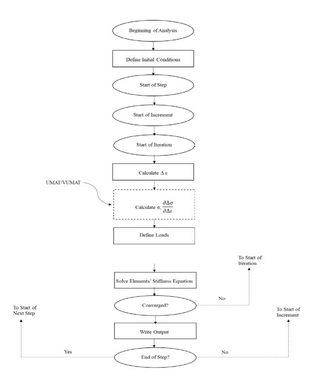
Figure 4.5 Abaqus Data Flow and Logic for VUMAT Subroutine
