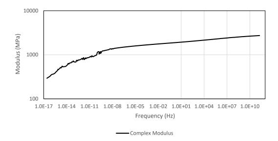
Figure 5.10 ANP Epoxy Complex Modulus Master Curve in Log-Log Plot
