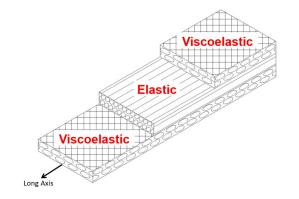
Figure 4.1 FlexLam Composite Laminate Layup
