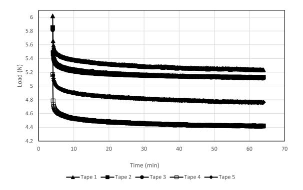
Figure 5.15 ANP Tape Springs One Hour Stowage Results Showing Loss in Tape Spring Deployment Force Over Time
