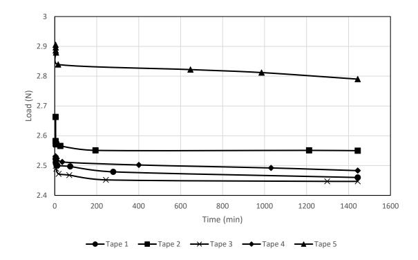
Figure 5.5 Control Tape Springs One Day Stowage Results Showing Loss in Tape Spring Deployment Force Over Time
