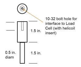
Figure 3.18 Dowel for Securing Tape Spring Tip During Structural Testing
