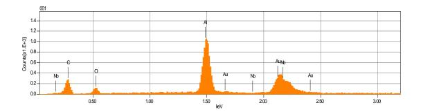
Figure 3.48 ANP Epoxy Element Composition (Point Analysis)
