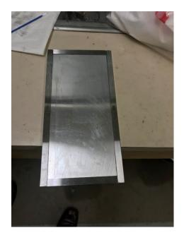
Figure 3.6 Mold for Neat Epoxy Sample
