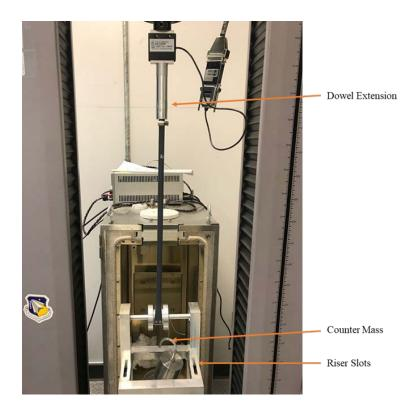
Figure 3.21 Structural Test Setup with Dowel Extension and Riser Slots
