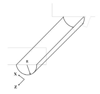
Figure 4.8 Pristine Tape Spring Shape and Global Coordinates
