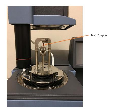
Figure 3.12 DMA Test on Neat Epoxy Coupon
