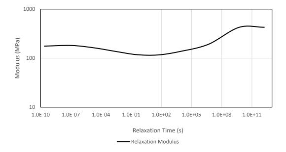
Figure 5.14 Prony Series Curve for Relaxation Modulus of ANP Epoxy in Log-Log Plot
