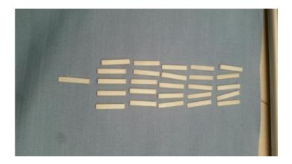
Figure 3.11 Neat Epoxy Coupons for DMA Testing
