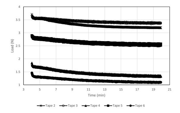
Figure 5.7 Control Tape Springs One Month Stowage (via TTSP) Results Showing Loss in Tape Spring Deployment Force Over Time
