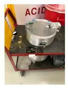
Figure 3.5 AFRL's De-Gassing Chamber
