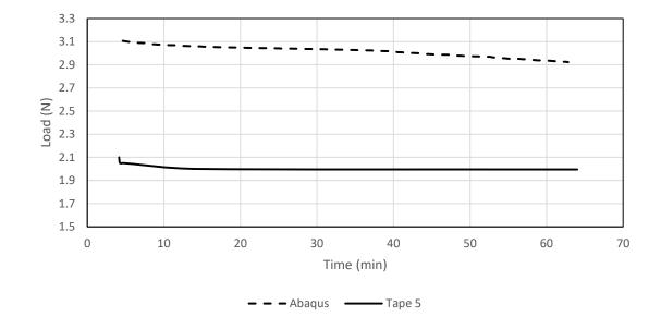
Figure 5.25 Comparison of Abaqus Predicted Results and Experimental Structural Test Results for Median Control Tape Spring (Tape 5) for One Hour Stowage
