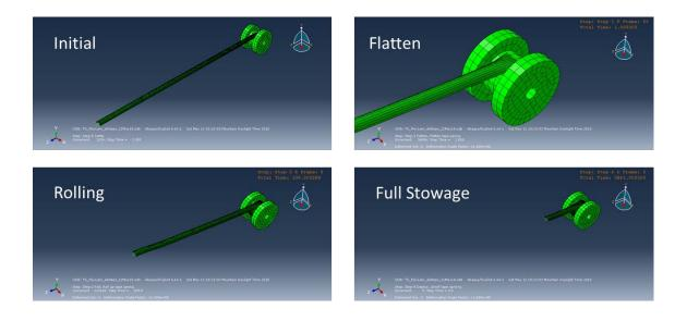
Figure 4.2 Tape Spring Simulation Steps in Abaqus
