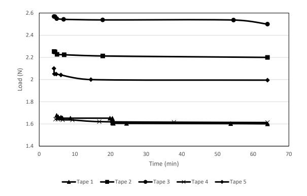
Figure 5.4 Control Tape Springs One Hour Stowage Results Showing Loss in Tape Spring Deployment Force Over Time
