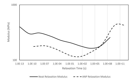
Figure 5.21 Comparison Between Neat Epoxy and ANP Epoxy Relaxation Modulus
