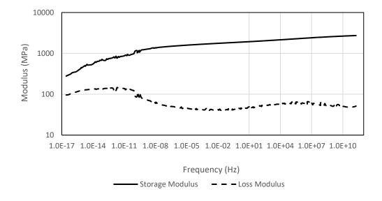
Figure 5.9 ANP Epoxy Storage and Loss Moduli in Log-Log Plot
