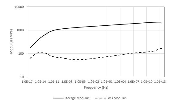
Figure 5.1 Neat Epoxy Storage and Loss Moduli as a Function of Frequency (Log Scale)
