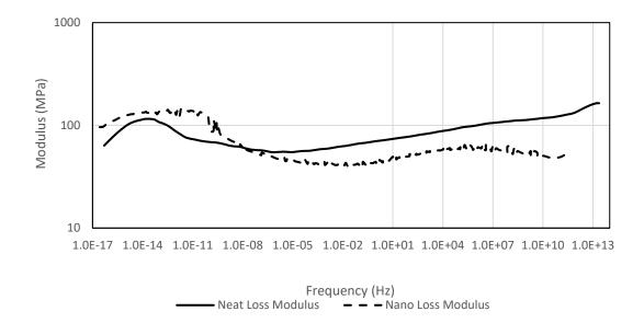
Figure 5.12 Neat Epoxy and ANP Epoxy Comparison of Loss Moduli in Log-Log Plot
