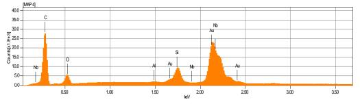
Figure 3.42 SEM/EDS Analysis of ANP Tape Spring
