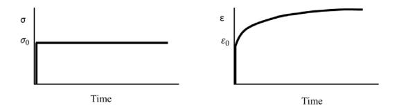
Figure 2.3 General Stress and Strain Behavior of a Material Subject to Creep
