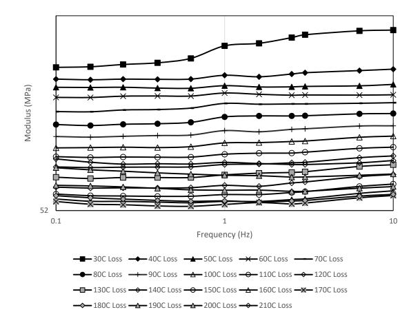
Figure 3.13a TTSP Data for Neat Epoxy DMA Tests, Loss Modulus – Trial #1 in Log-Log Plot
