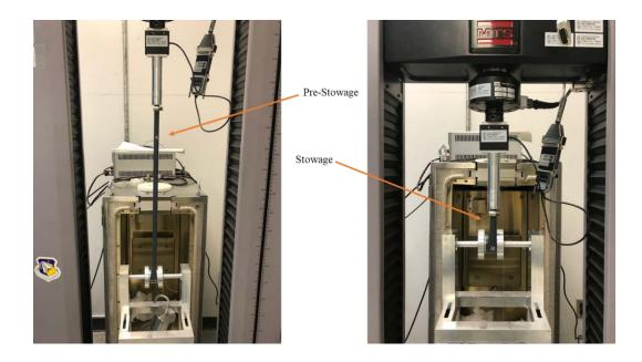
Figure 3.23 Structural Test Configuration for One Hour and One Day Tape Springs
