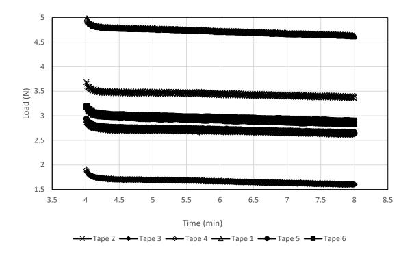
Figure 5.6 Control Tape Springs One Week Stowage (via TTSP) Results Showing Loss in Tape Spring Deployment Force Over Time
