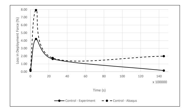
Figure 5.36 Abaqus vs Experimental Tape Spring Tip Deployment Force Loss for Control Tape Springs
