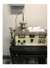
Figure 3.35 SEM Coating Machine
