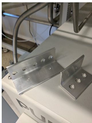
(a) Brackets used to connect the wire leads
