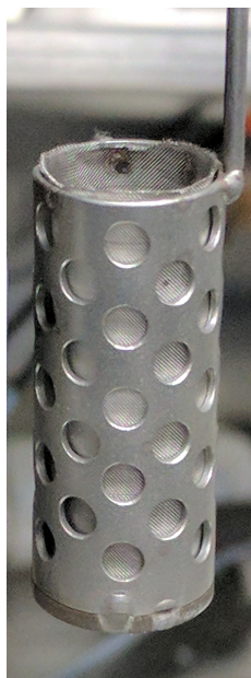
Figure 5.10: Photograph of first anode basket design
