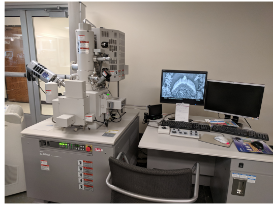
(b) Hitachi S-4800 Field Emission SEM with Energy Dispersive X-ray Spectroscopy
