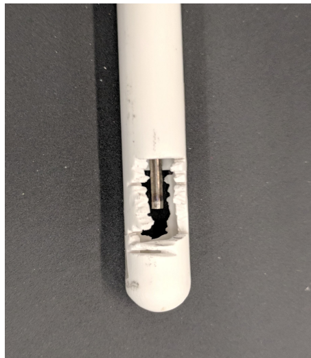
Figure 5.11: Photograph of custom mullite tube basket
