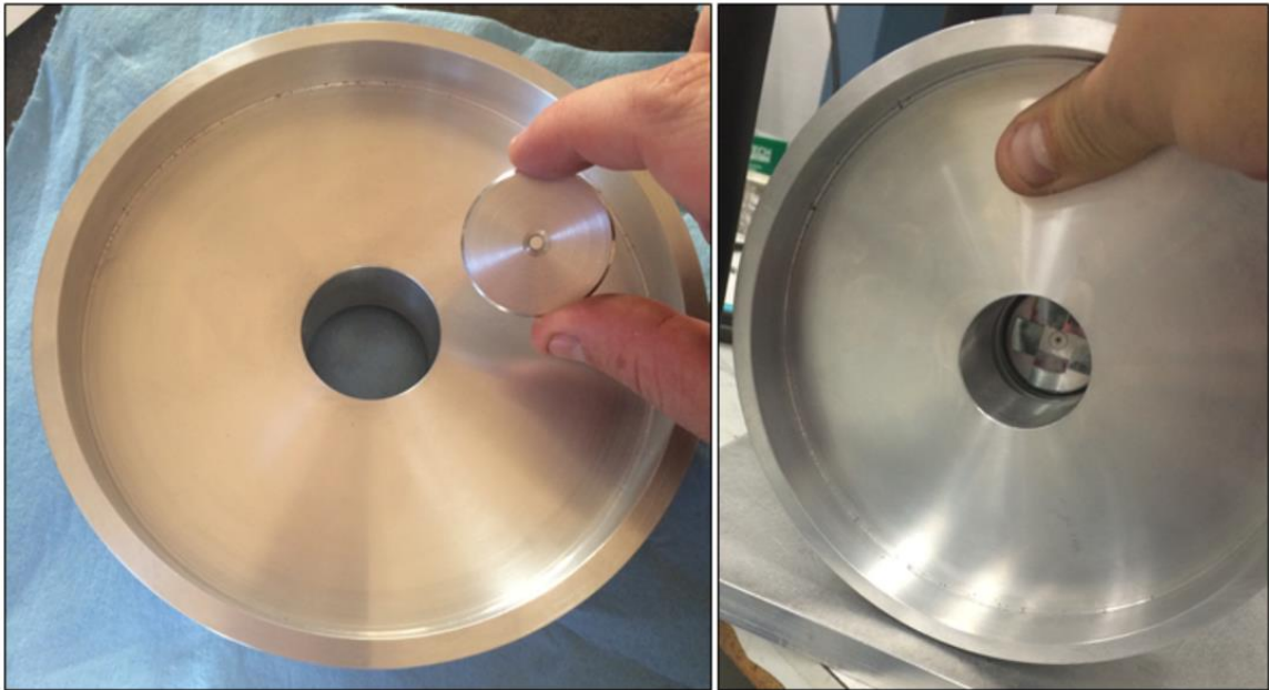
Figure 3.13: Alignment plate used to mate cryostat to proton beam.
