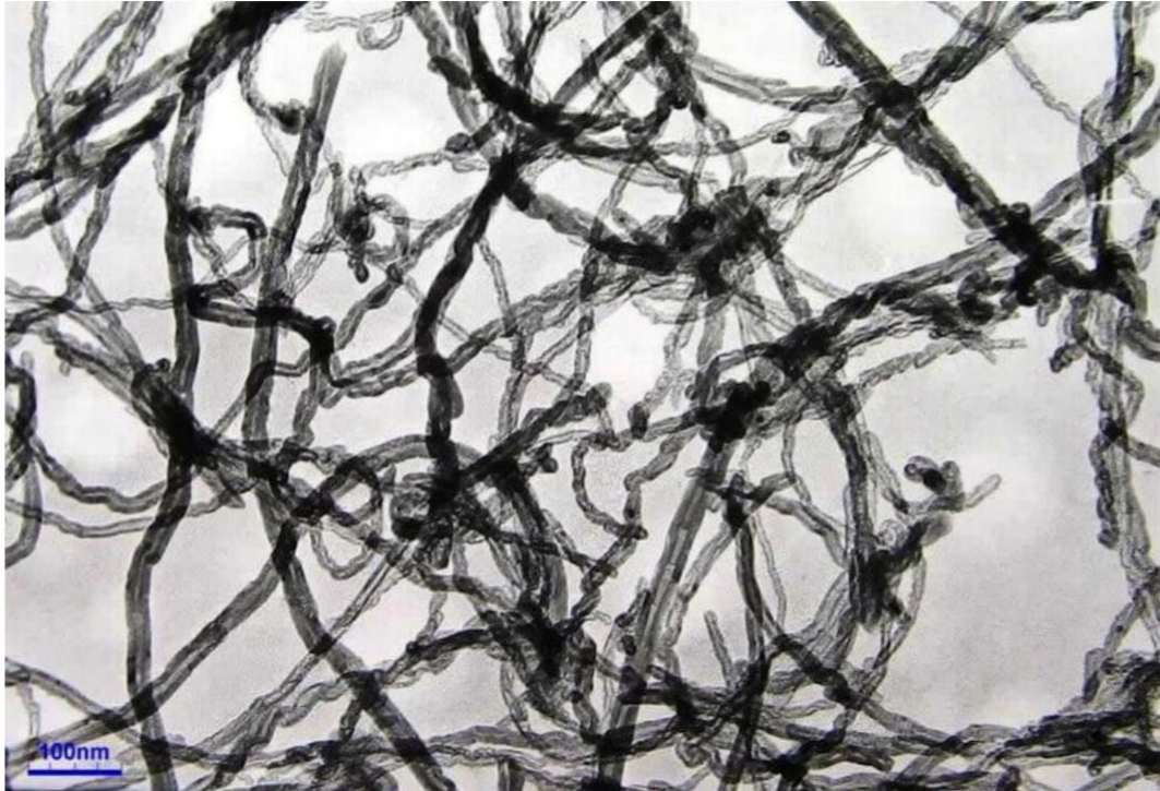
Figure 3.2: Transmission electron microscope (TEM) images of MWCNTs.
