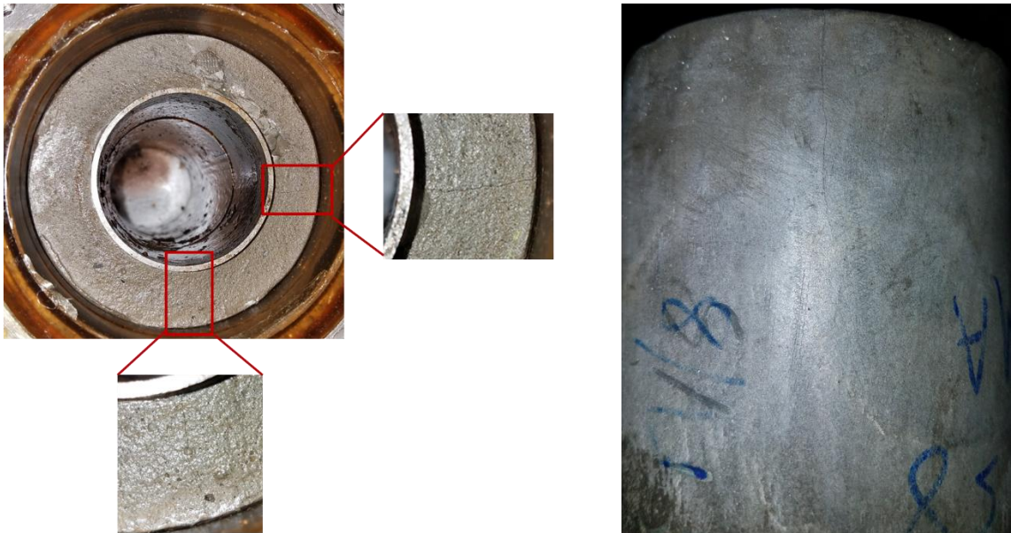
Figure 3.60: Post cyclic test integrated seal specimen sealed with NM-MMA showing two longitudinal cracks in the cement sheath.
