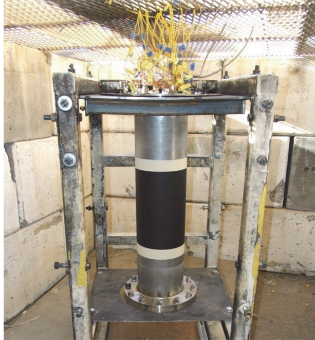
Figure 7.7: Instrumented pressure vessel mounted in the test fixture
