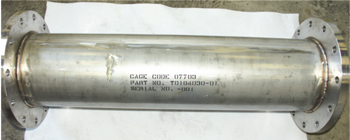
Figure 7.5: Example of one of the cylinders after rolling and welding without the end caps attached
