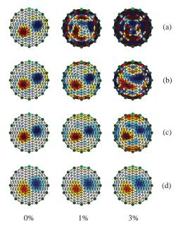
**Figure 1:** Image reconstructions. (a) Standard GN method; (b) Electrode movement model; (c) Proposed method with  $\mu = 1$  and  $\tau = 1$ ; (d) Proposed method with  $\mu = \sqrt{0.1}$  and  $\tau = 0.1$ . From left to right, distortion amplitude increases from 0%, 1% to 3% of model diameter respectively.
