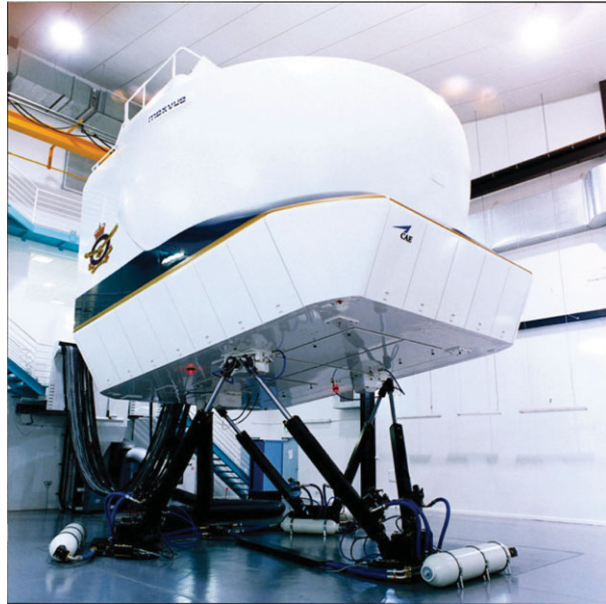
Fig. 1. (Colour online) CAE's version of the Gough–Stewart motion platform for a flight simulator.
