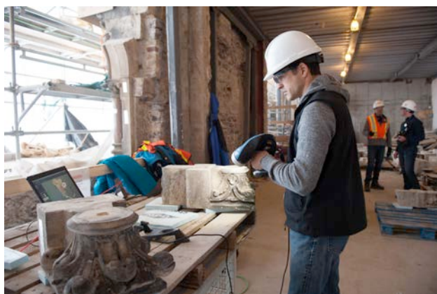
Figure 1. Data capture with a Creaform HandySCAN 3D handheld scanner.
