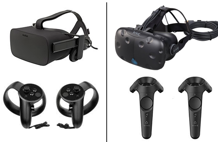
Figure 1.1: Two of the most popular Head Mounted Displays (HDMS) and their controllers: Oculus Rift (left) and HTC Vive (right).
