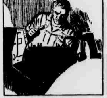
With the Combination Mirror and Trouble Lamp You Can Find That Lost Nut or Broken Part.
