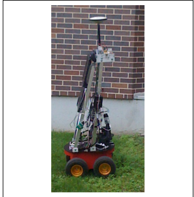
Figure 7. Pioneer rover with tilt unit and LiDAR attached. LiDAR: light detection and ranging.
