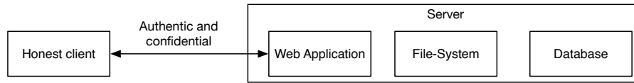
Fig. 5.1: The communication model between the honest client, the web application, the file-system and the database
