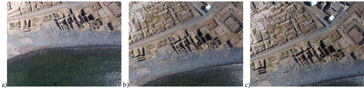
Figure 5. Irregular overlap clearly visible in three consecutive images of the same strip from the Nora dataset (Flight 1).
