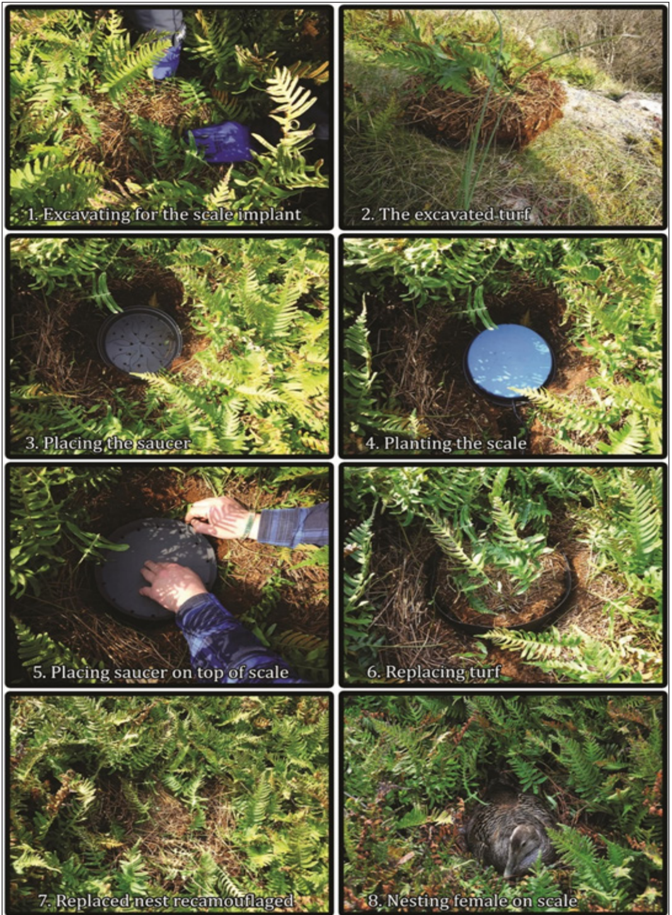
Figure S1. The implant of the automatic poultry scale systems. The scales were implanted in the pre-incubation period.
