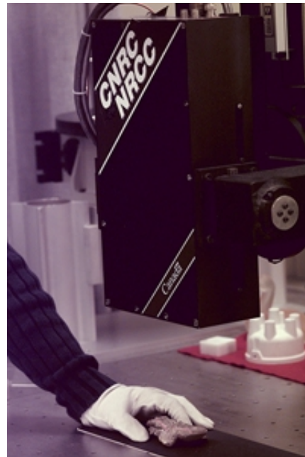
Figure 2. Laser unit of 3D scanner developed by the division of Visual Information Technology, National Research Council Canada.
