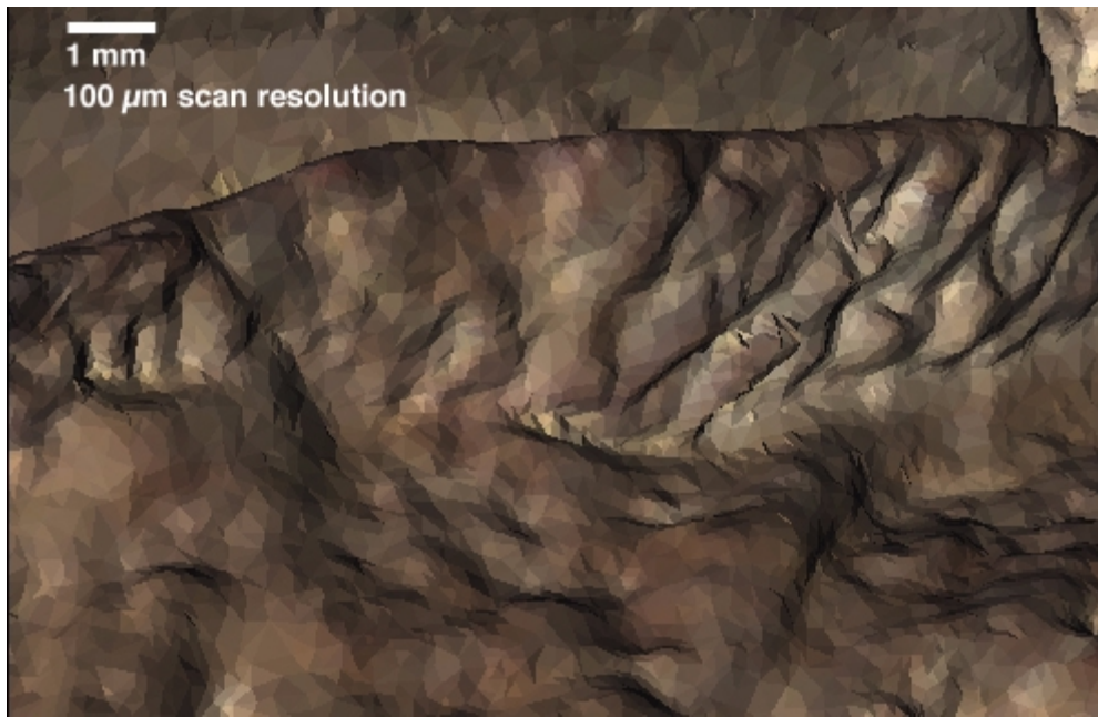
Figure 9. Magnification of 3D 100 µm resolution scan from 800,000 polygon Tylosaurus sp. basisphenoid-basioccipital model illustrating faceting.
