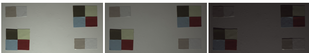
Figure 14: Three images of a MLIC capture of a planar surface with flat paper targets with different albedo regions.
