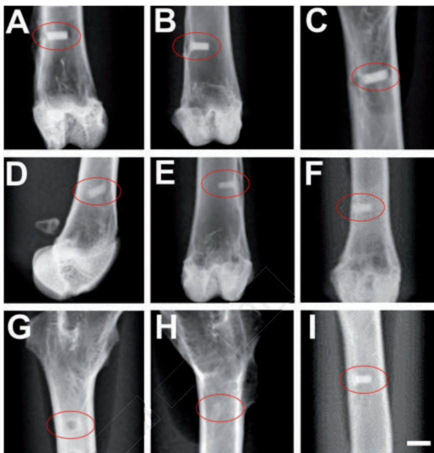
Figure 2. X-rays: antero-posterior and lateral side of femurs of three treatments (C cement in top row, P cement in middle row, PG cement in the bottom row) to 1 month (left column), 6 months (middle column) and 12 months (right column). Radiographs showed good images and maintenance of the samples in the original implant areas (red circles) in all different times and for all three types of cements. Only the radiographic images of PG cement at 6 months do not show sufficiently the implant (image H). Scale bar: 1 cm.
