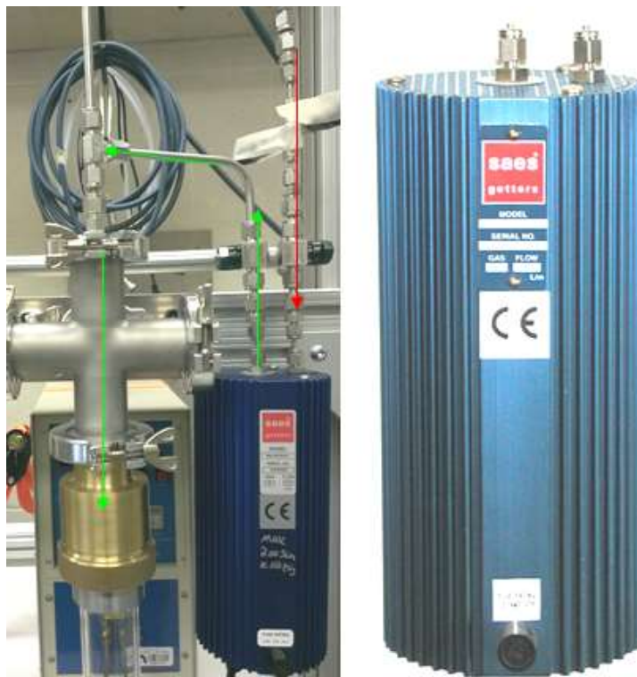
Figure 3.4: Left: Heated argon purifier and Ar delivery manifold. Ultra high purity argon is delivered from a gas bottle to the inlet of the purifier (red arrow). The purifier removes residual gasses, such as nitrogen and oxygen, before flowing into the vacuum chamber (green arrows). Right: Closeup of the SAES GC50 heater argon purifier.
