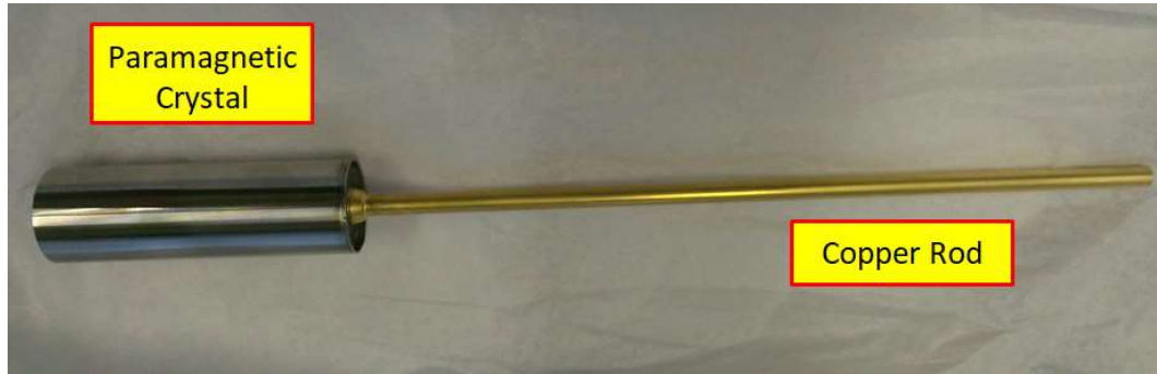
Figure 7.5: A photograph of a paramagnetic crystal canister outside of the ADR magnet bore. The crystal material is housed within the stainless steel canister and the gold plated copper rod extends past the magnet bore to allow attachment of experiments. A wires brush of 100 wires inside the canister are used to make thermal contact from the crystal within to the copper rod.
