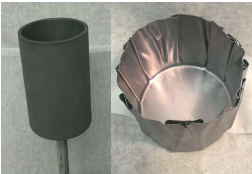
Figure 3.5: Left: 1.25" diameter graphite susceptor, with a machined well to house samples. Right: 1.125" diameter tantalum cup stamped from 0.005" thick tantalum foil. The tantalum acts as a liner between samples and the graphite crucible.
