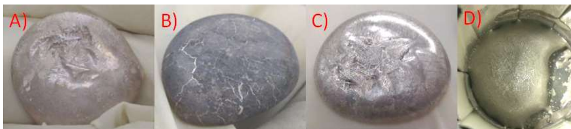
Figure 3.10: Various intermediate samples created during refinement of the Ag:Er paramagnet recipe. A) Erbium oxide (pink) and B) erbium nitride (black) which led to the use of purified argon. C) Erbium carbide (brown) which led to the use a tantalum cup insert in the graphite susceptor. D) silver erbium 1:1 intermetallic (matte tan) forced the melting temperature to be above 1226° C while stirring.
