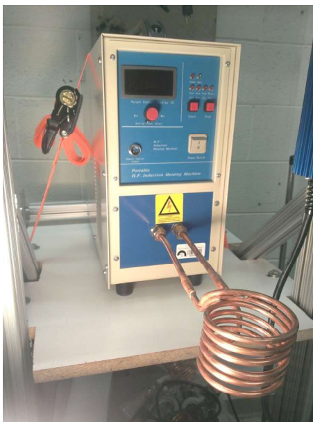
Figure 3.2: Close up view of the induction heater unit and the copper heating coils. A quartz tube, not pictured here, that acts as the vacuum and sample chamber is placed within the coils.
