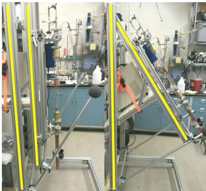
Figure 3.7: Profile photographs of the support frame and system. Left: the system in its usual vertical position. Right: The system tilted to 30 degrees. The combination of tilt and sample rotation allows for a “cement mixing” action of molten samples. Yellow lines are drawn to guide the eye.
