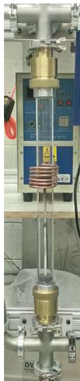
Figure 3.3: Photograph of the clear quartz tube that is used as the vacuum chamber for paramagnetic alloy preparation. The tube sits within the coils of the induction heater and its non-conductive nature allows the induction power to pass into the vacuum space uninhibited. The quartz tube is sealed at both ends with brass couplings that attach to the vacuum pumping lines (below) and argon gas delivery manifold (above) via KF-40 joints.
