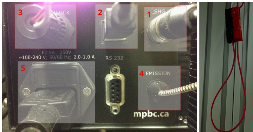
Figure 2.38: MPBC laser box, back panel. On the left: Number 1 connects the control box to the collimation box and produces the control signals. Number 2 connects the control box to the back of the computer and is a USB connection for computer-based control. Number 3 is the interlock, number 4 is the emission fiber, and number 5 is the power strip. On the right: the interlock from the left figure. Interlock needs to be connected as shown here. The wires at the top of the figure are the same ones that come out of the interlock in the left image.
