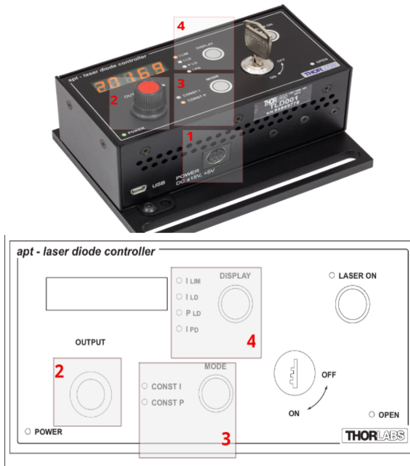
Figure 2.39: Laser controller TLD001. Number 1 is the power connection, number 2 is the output potentiometer and is used to set the output intensity (power) of the laser, number 3 switches between constant power and constant current modes, number 4 can be set to show one of 4 operating parameters as follows: I_{LIM} for the maximum drive current limit, I_{LD} for the laser diode drive current in mA, P_{LD} for the laser diode optical output power in mW, and I_{PD} for the photo diode current in mA. This figure is taken from [6].
