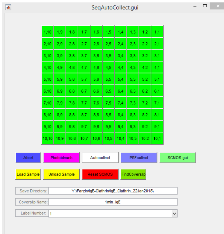
Figure 2.46: Sequential microscope GUI. Each green button on the grid takes us to a specific location on use of the stepper motor.
