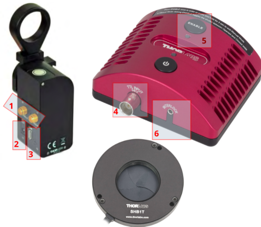
Figure 2.12: Flip mount and shutter for 647 laser beam control. Number 1 shows two SMA connectors, marked DIG I/O 1 and DIG I/O 2, for use in applications requiring an external trigger in form of a TTL signal to toggle flipper position. Number 2 is power supply connection. Number 3 is USB connector for the computer. Number 4 shows the TTL connector for the shutter controller. Number 5 is mode button to enable the shutter controller for either manual or computer based control. Number 6 is the interlock. This figure is taken from [3].
