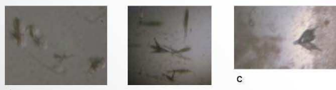
Fig.7 BAAT C235A microcrystals obtained with 0.1M HEPES pH 7.5, 10% PEG 6000, 8% ethylene glycol as precipitant. A) apo-protein, B) in presence of 5 mM stearyl-CoA. C) Crystals of wild type BAAT in presence of 1 mM sodium cholate, 1 mM CoA obtained with 0.2M calcium acetate hydrate, 0.1M sodium cacodylate pH 6.5, 18% PEG 6000.
