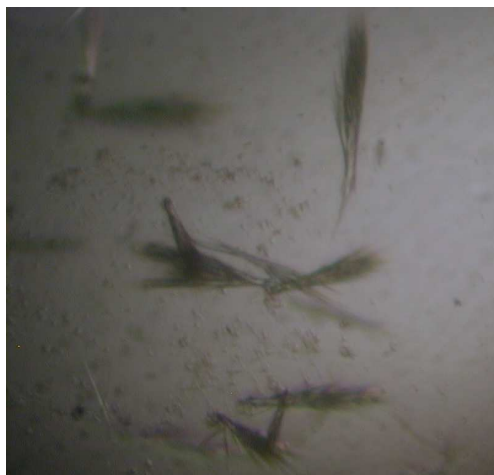
Fig.3.15. BAAT C235A microcrystals obtained with 0.1M HEPES pH 7.5, 10% PEG 8000, 8% ethyleneglycol as precipitants.
