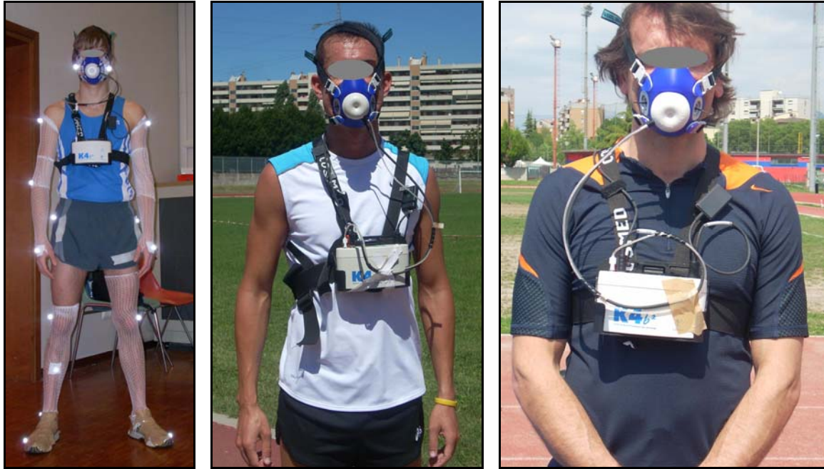
Figure 19.1. K4b 2 during experiments on the treadmill (on the left) and in the track (on the right).
