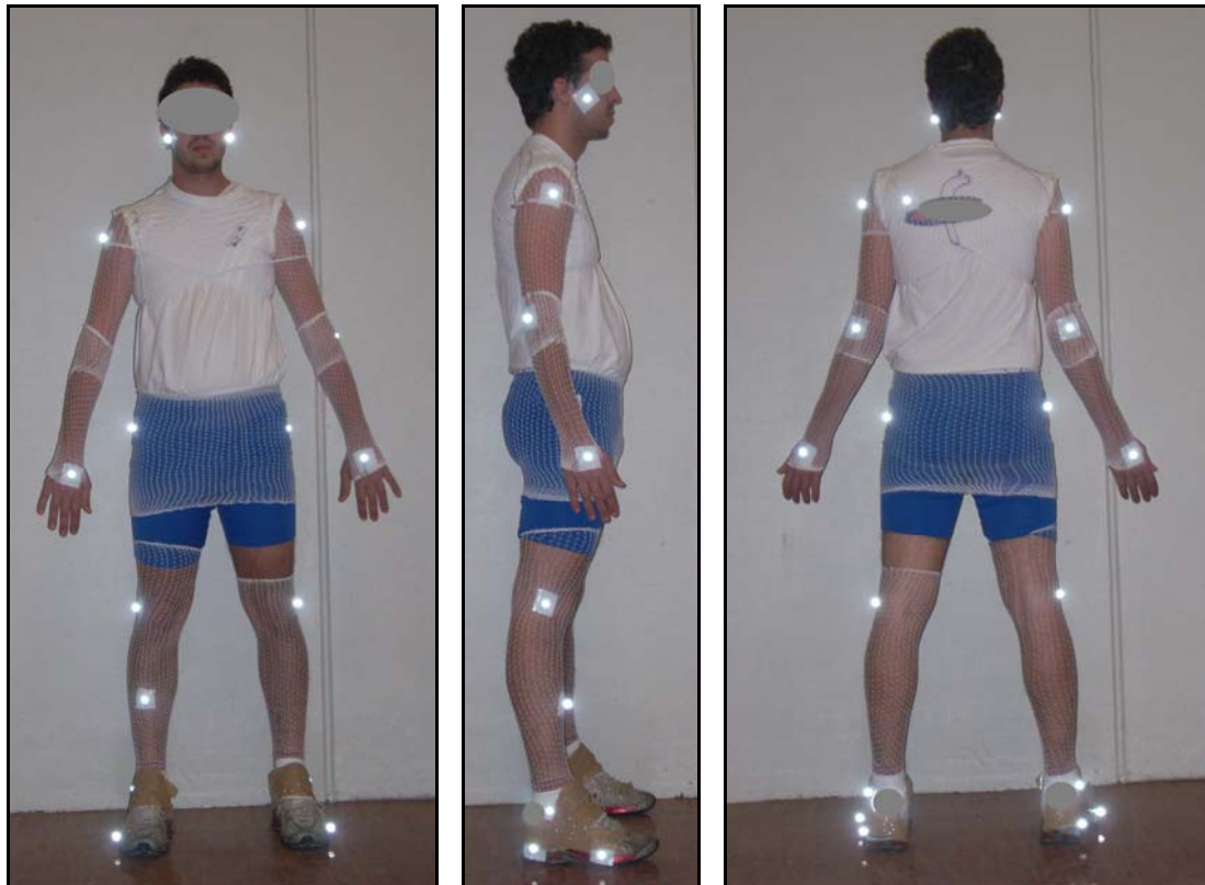
Figure 5.1. Markers placed on a subject
