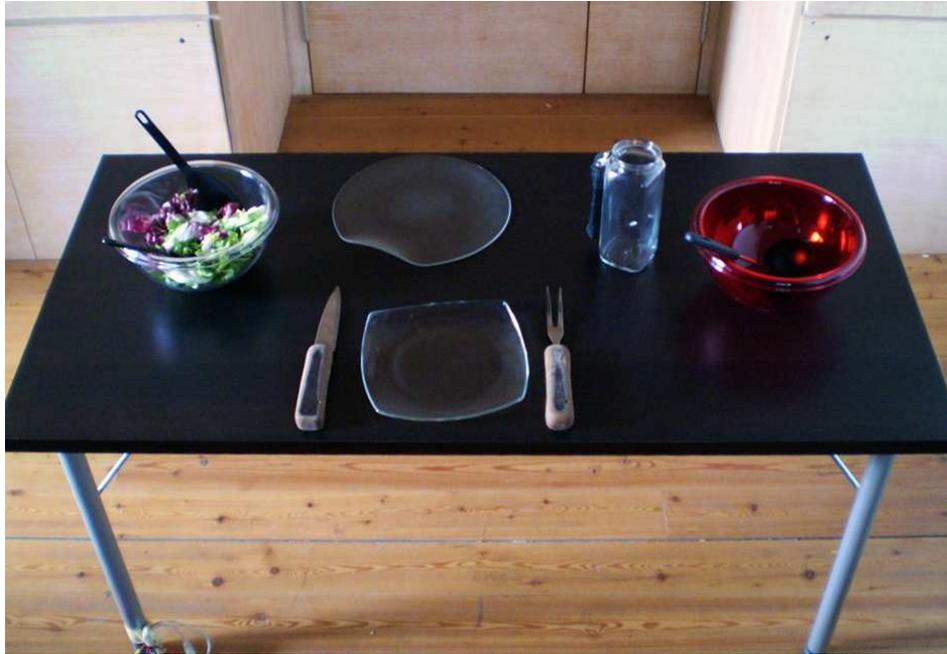
**Fig. 3.1.** The final prototype of the Gamelunch. Various sensors are embedded in both the table and kitchenware. Loudspeakers for sound feedback are embedded in custom-made holes under the table.
