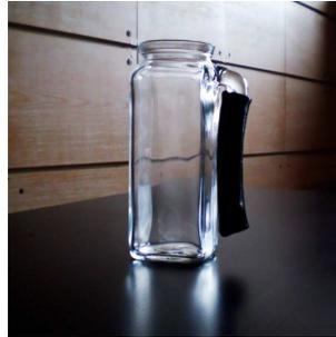
(b) The jug. A board from a Wii Remote is embedded into the handle and covered with rubber.
