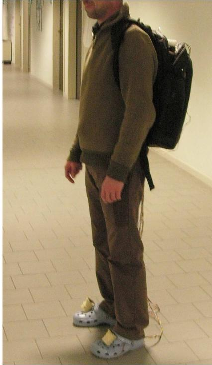
**Fig. 3.9.** The complete interface, with the early version shoes prototype. The backpack hosts a laptop and an acquisition board which senses data from the shoes. These data drive a set of real-time physically-based models running on the laptop and providing low-latency audio feedback through the shoe-mounted speakers.
