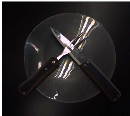
(c) Fork and knife, laid on a glass dish. A force sensor is embedded into the table below the dish, sensing the pressure exerted on it.
