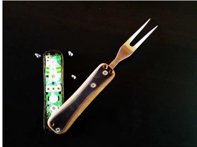
(a) The fork, opened up in order to show the embedded board which is taken from a Wii Remote controller.
