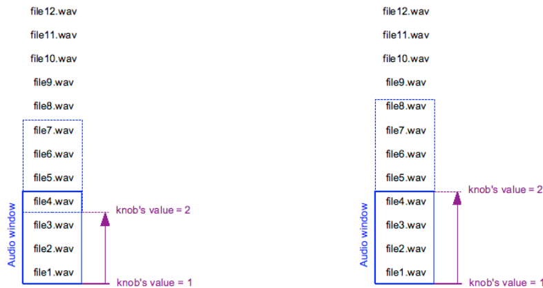
Fig. 6.6. Four sound files are simultaneously processed in the DWM and the increment of the knob's value enables to move the mesh 3 sound files forward (left figure) or 4 sound files forward (right figure).
