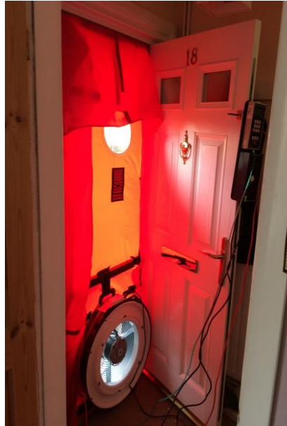
Figure 8: The setup of blower-door at House No.4
