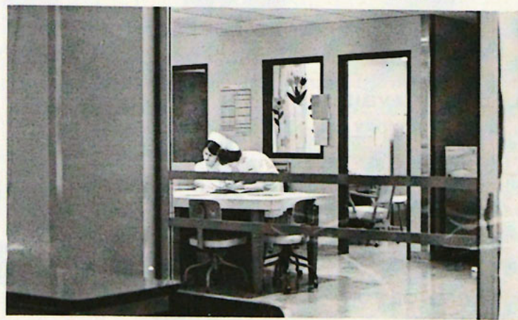
A PATIENT'S EYE VIEW OF ICU, SHOWS THE SLIDING GLASS DOORS, THE HEAD NURSE OFFICE (CENTER), AND THE NURSES DESK TO THE LEFT. THE DESK IS SITUATED SO THAT VISUAL OBSERVATION OF EACH PATIENT ROOM IS POSSIBLE.
