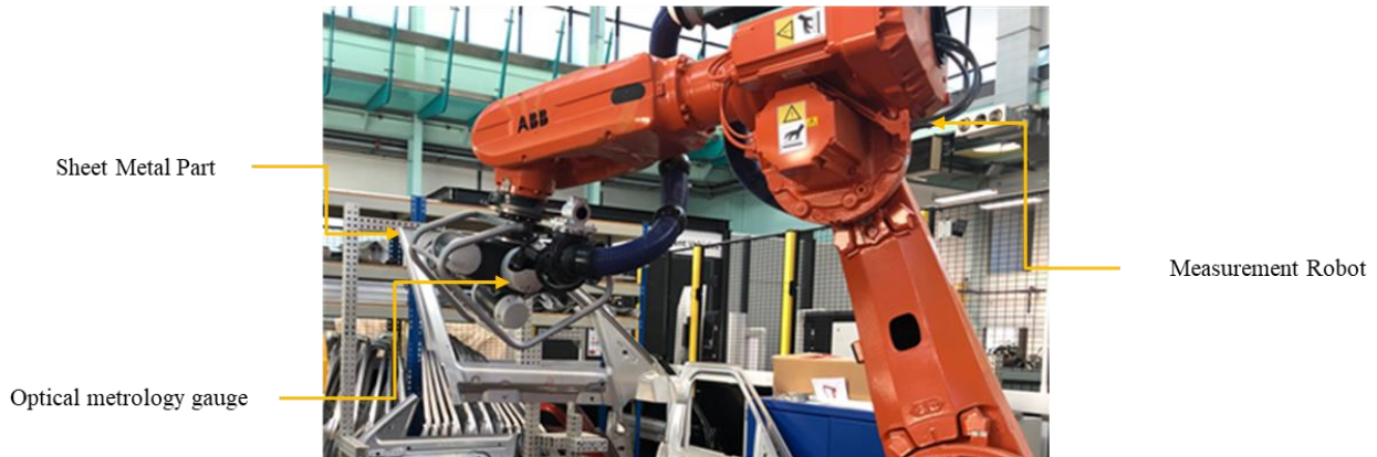
Figure 1. An automatic optical metrology gauge mounted as end-effector on the robot (3D optical scanner)
