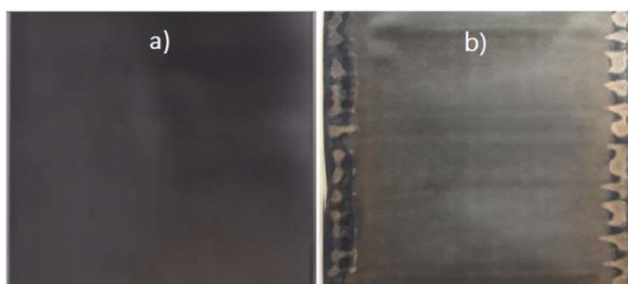
Figure 7: Photographs of graphite electrodes: a) new cell and b) Set A cell
