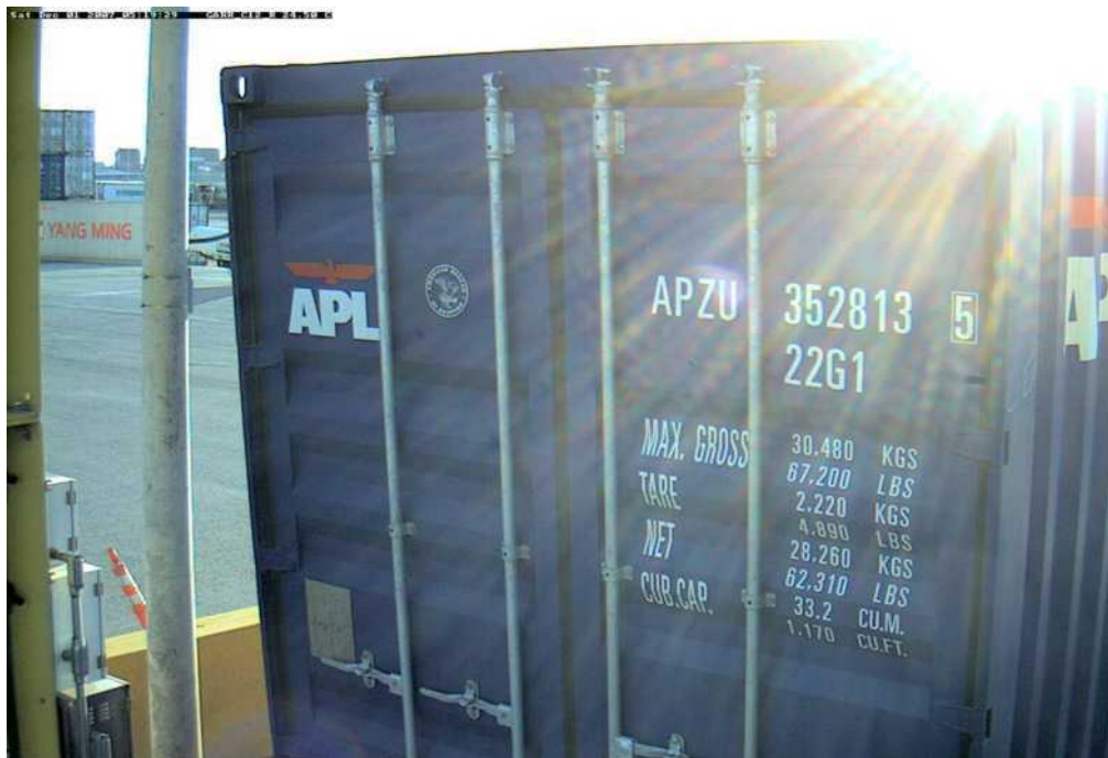
Figure 3: Example of Sun Negatively Impacting Image Quality
