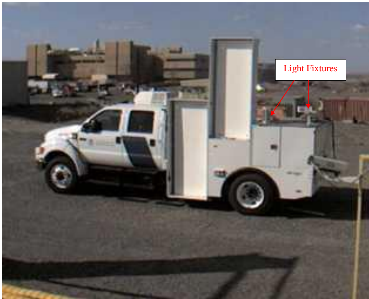
Figure 22: Location of Light Fixtures Mounted on Roof of the Mobile RPM
