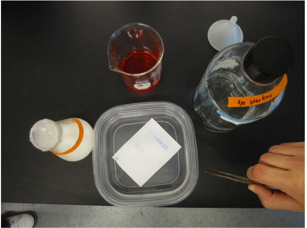
Figure 2. Preparation of the nitrocellulose membrane for antibody staining with marker lane on the right in blue and cell line in center with orange tint.
