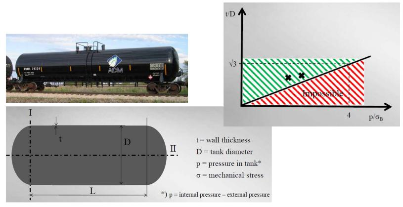
If the mechanical stress in the tank equals the fracture stress  $\sigma B$ , we can derive the non-dimensional relationship t/D =  $(\sqrt{3}/4) \cdot p/\sigma B$
