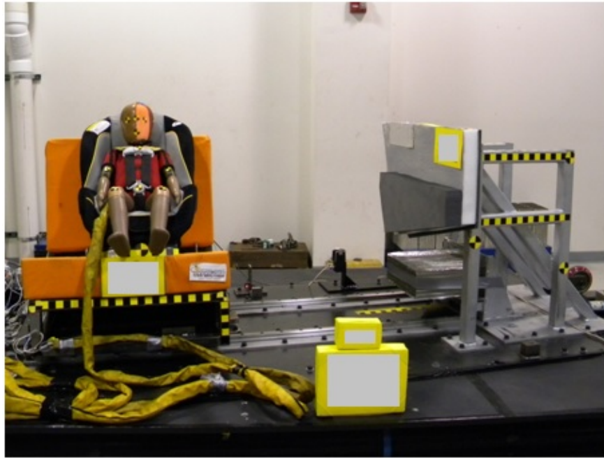
Figure B1: Front view of side impact fixture attached to the deceleration sled
