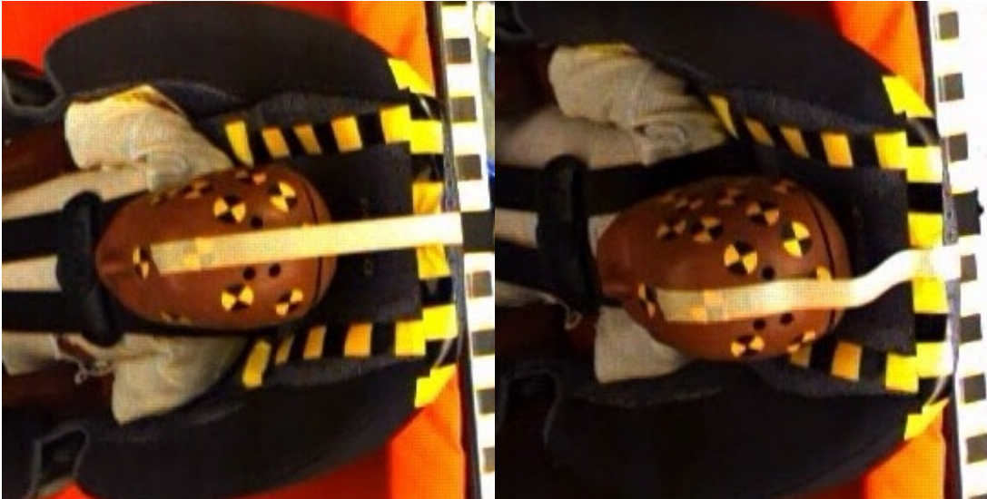
Figure 15: Overhead still photos from high-speed video depicting maximum forward and rearward movement of taped ATD head
