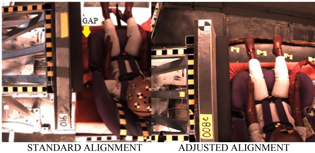
Figure 32: Overhead view of CRS-to-door interface at impact with the aluminum honeycomb
