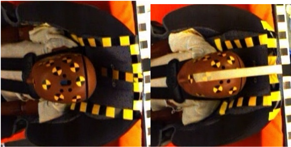
Figure 14: Overhead still photos from high-speed video depicting maximum forward movement of untaped and taped ATD head
