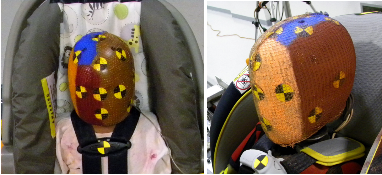
Figure B4: CRABI 12 and Q3s heads prepared for testing with targets, copper mesh cover, and test chalk
