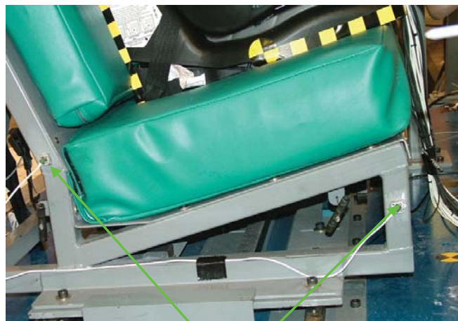
Accels in X- and Y-axis on sliding seat (primary and redundant)
