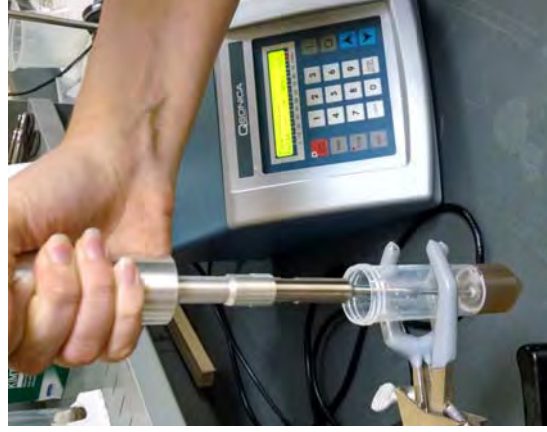
Figure 1: Sonication of microbubble-nanoparticle mixture with 3 mm probe driven at 20 kHz.
