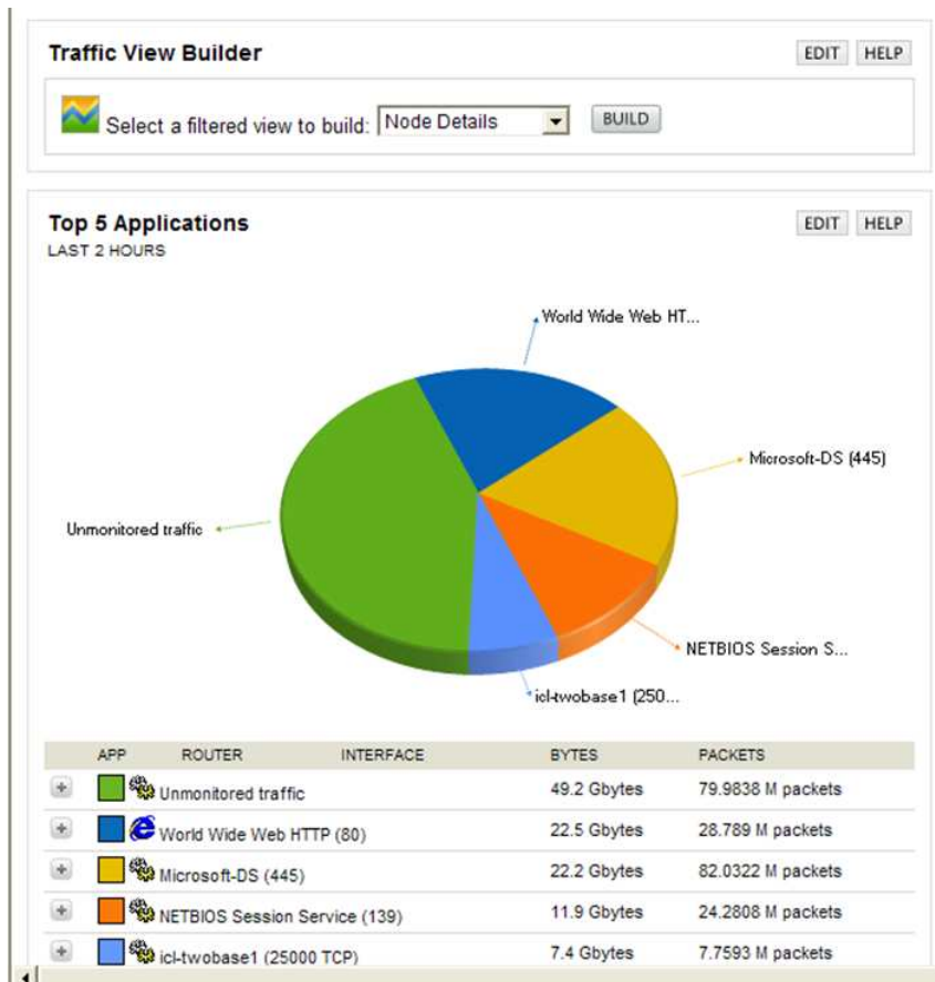
Fig 8A - from Orion Solarwinds diagram of the top 5 talkers on the network in almost live time. This example illustrates HTTP web traffic as the top throughput.
