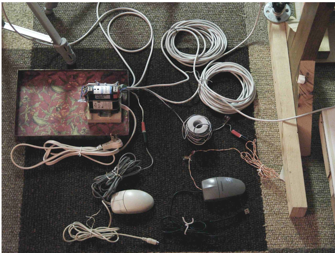
Laser Relay Box and Mouse Connections for both Reaction Time and Balance Testing
