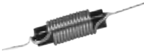
solenoidal wound inductor
