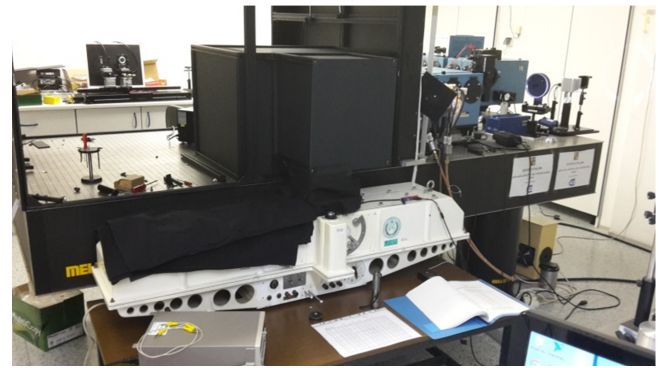
Figure 3. Photo of the CMI measurement setup. Double-grating monochromator is on the left side, the output optics light-tight box in the middle of the picture as well as the Dobson 074.
