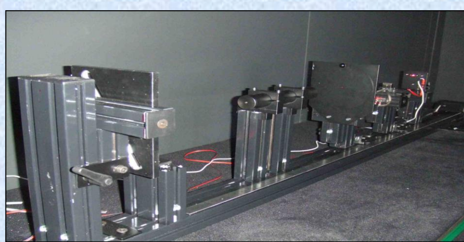
Picture 3. Horizontal Absolute Irradiance Calibration Set-up
