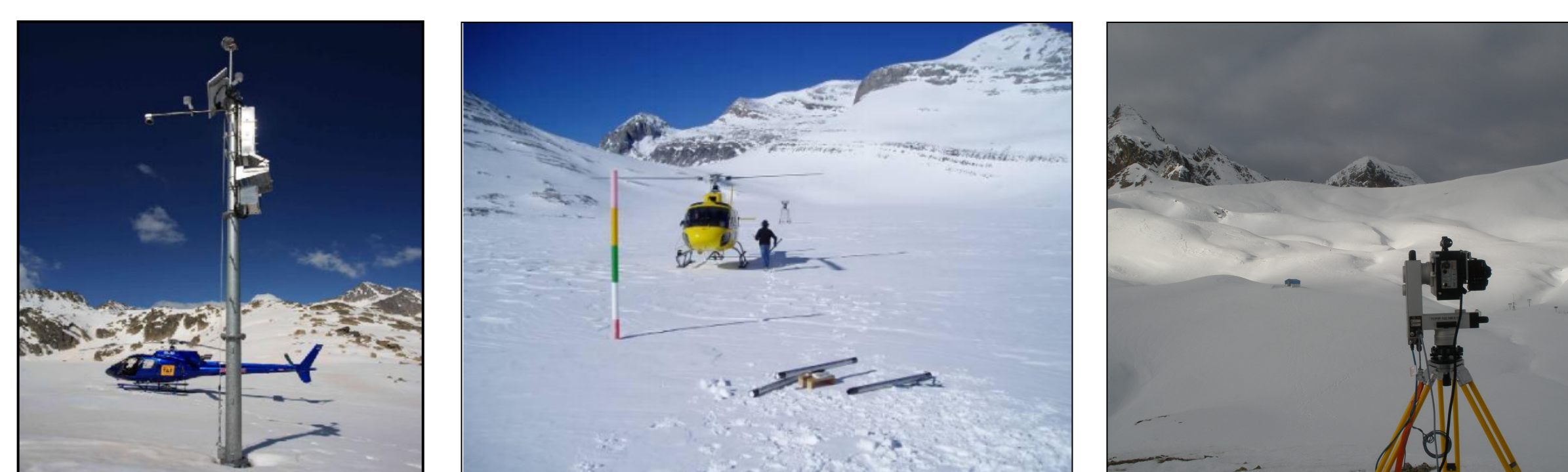
Figure 5: Sources of information in snow cover and depth in the Pyrenees. The telenivometer (left) measures depth and density of snow, same as the manual measures (center), while TLS (right) is used to measure complete areas.
