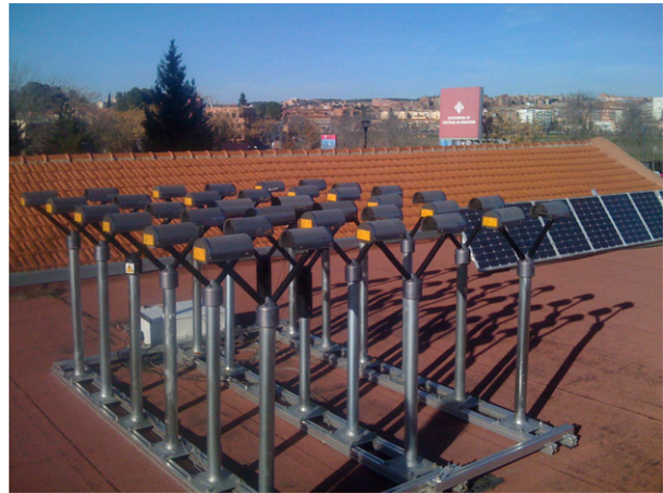
FIG. 1. Setup of the experiment: 18 laser disdrometers collocated as close as possible (Toledo, Spain). The instruments at the center are two Parsivel-2 instruments that were not used for this experiment. The two Parsivel-1 instruments most uncorrelated with the rest were not used for the calculations, resulting in the experiment based in 14 disdrometers.
