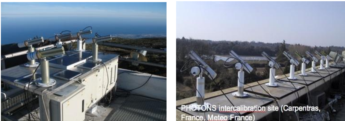
Fig. 5 . (a) Izana (INM, 2440 m a.s.l) for Reference or Master instrument ; (b) Carpentras (Météofrance) for inter-calibration against Reference instrument.
