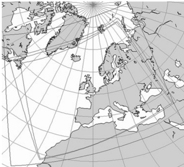
Fig. 2. Integration areas for the limited-area models used in GLAMEPS. Outer area: output domain for data from EuroTEPS in model levels; Medium area: ALADIN domain with extension zones; Inner area: HIRLAM domain and output domain for common products.
