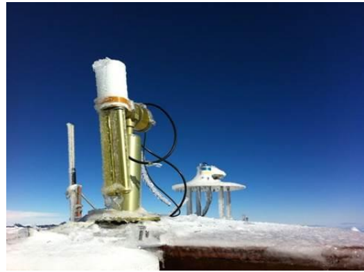
Figure 9.2. Cimel at Teide Peak Observatory, blocked by ice.
