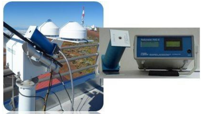
Figure 10.5. Absolute cavity radiometer (PMO6) installed at IZO during summer 2014 in the sun-tracker of the BSRN.
