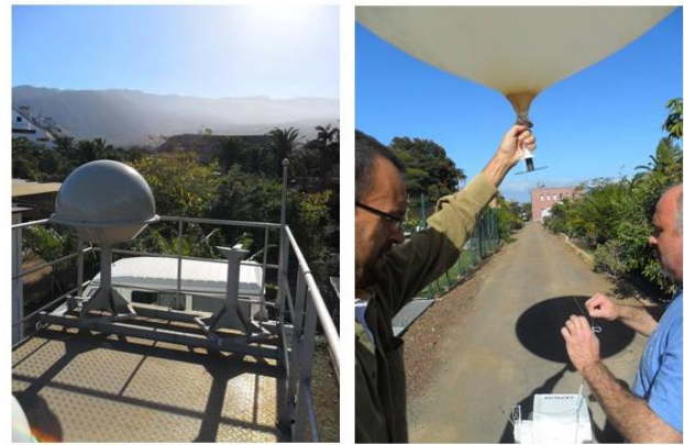
Figure 5.2. Ozonesonde station located at BTO (left), and moment of balloon release (right).
