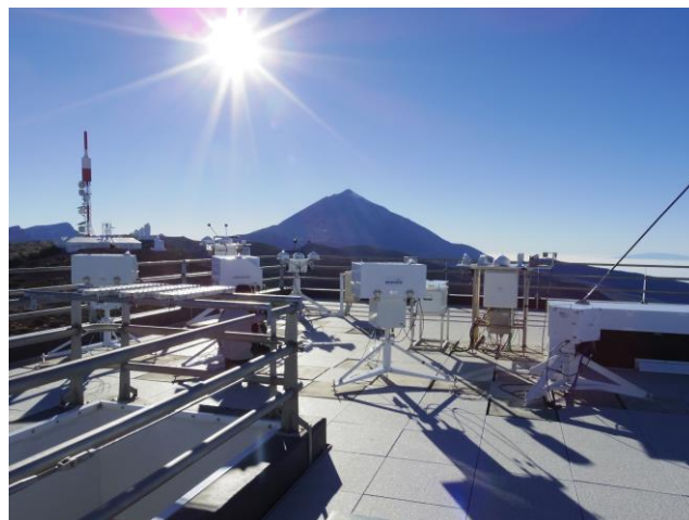
Figure 17.1. RBCC-E Brewer spectrophotometer triad located at Izaña Atmospheric Observatory (Photo: Alberto Redondas).
