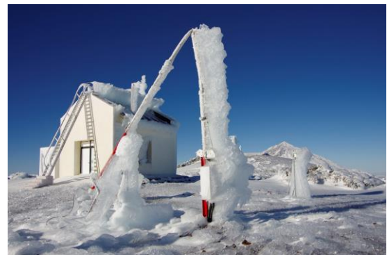
Figure 13.6. Hard rime affecting IZO weather station after the storm from 15 to 18 February 2014. We can see the steel mast of one of the weather stations, broken in half (Photo: Rubén del Campo Hernández).
