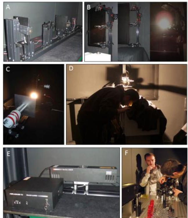
Figure 3.5. Images of the IZO Optical calibration facility. A) Horizontal absolute irradiance calibration set up, B) Three stages of a Brewer irradiance calibration with the vertical set up, C) Absolute radiance calibration of a Cimel CE318, D) Angular response function determination of a Brewer (Photo: Alberto Redondas), E) Set up for Slit function determination and F) Alignment of a Brewer spectrophotometer optics (Photo: Alberto Redondas).
