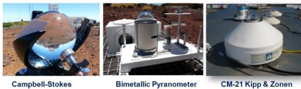
Figure 10.6. Campbell-Stokes sunshine recorder, bimetallic pyranometer, and Kipp & Zonen CM-21 pyranometer installed currently at IZO during the one-year intercomparison.
