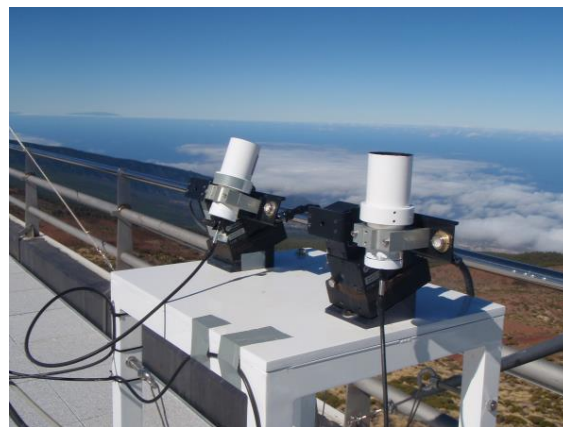
Figure 11.2. DOAS instruments outdoor optics with sky trackers.
