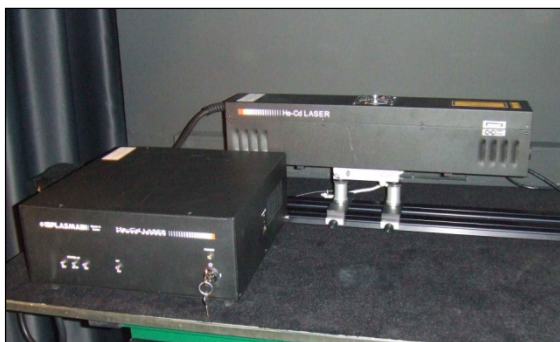
Fig. 6. Slit function determination set-up.
