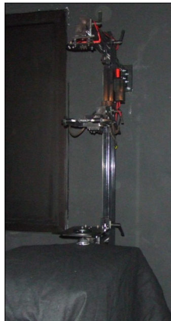
Fig. 2. Vertical absolute irradiance calibration set-up.
