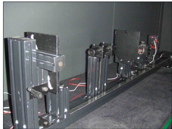
Fig. 1. Horizontal absolute irradiance calibration set-up.
