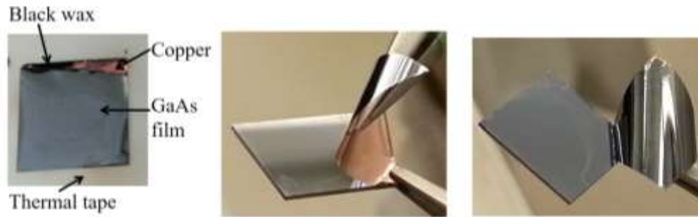
Figure 2.24: Copper and GaAs protective layers result in better thin films
