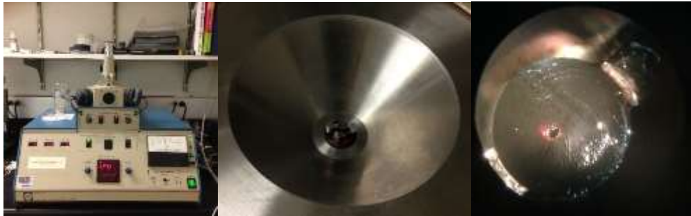
Figure 4.2: Top: Ion Mill Wedge Calculations diagram. Bottom: Ion Mill (left), Cz silicon specimen on holder and in ion mill bay (center), View of perforation through ion mill microscope (right)
