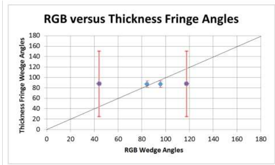
Figure 3.20: Comparison of thickness from RGB and Fringe method for areas 5046 and 5047 in specimen GKF 044-14. Original image data in purple, and grey-removed data in blue.
