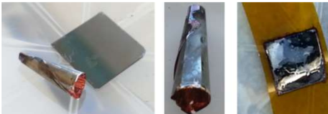
Figure 2.21: Problems with GaSb films- cracking and oxidation
