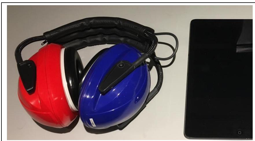
Figure 2. Creare wireless automated hearing test system including iPad.
