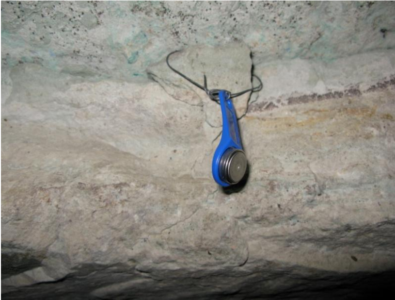
Figure 3. Photograph of an iButton Hygrochron temperature and relative humidity data logger deployed in a M. thysanodes maternity roost site (Photo by L. Bonewell).
