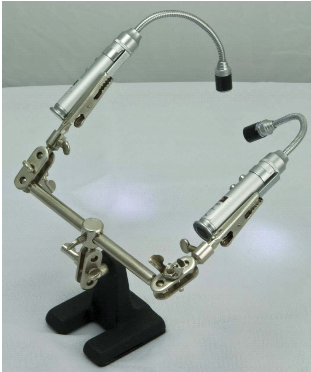
Figure 21. Lighting setup for illuminating microscopic subjects.
