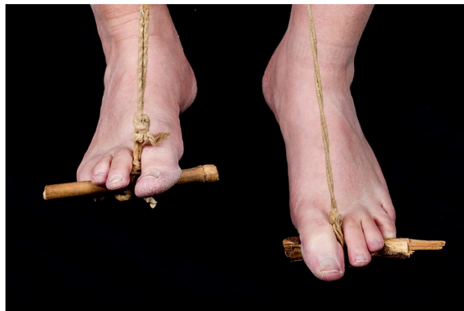
Figure 41. Weaver places his toes between the cords and alternately press downward to cause the shafts to move up or down. Photograph by Tom Crosman.
