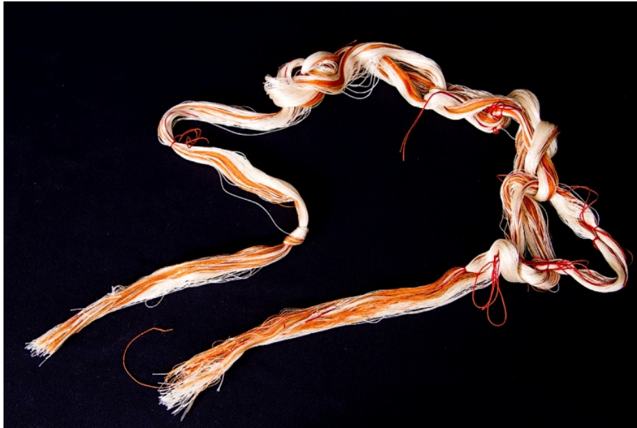
Figure 17. Warp that has been measured, cut, and removed from a warping board and ready to place on the loom. Photograph by Tom Crosman.
