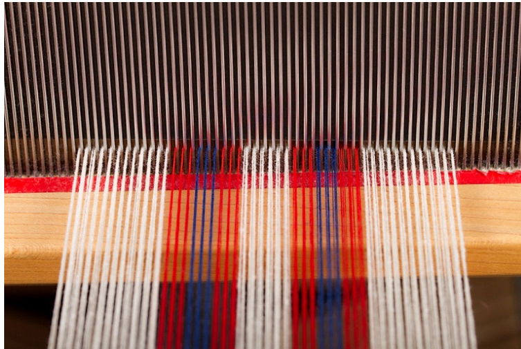
Figure 21. Close-up of a reed, the metal piece consisting of many slots called dents. One function of the reed is to keep the warp threads straight and parallel to each other when weaving. Reed and beater work together to beat the weft in place. Photograph by Tom Crosman.
