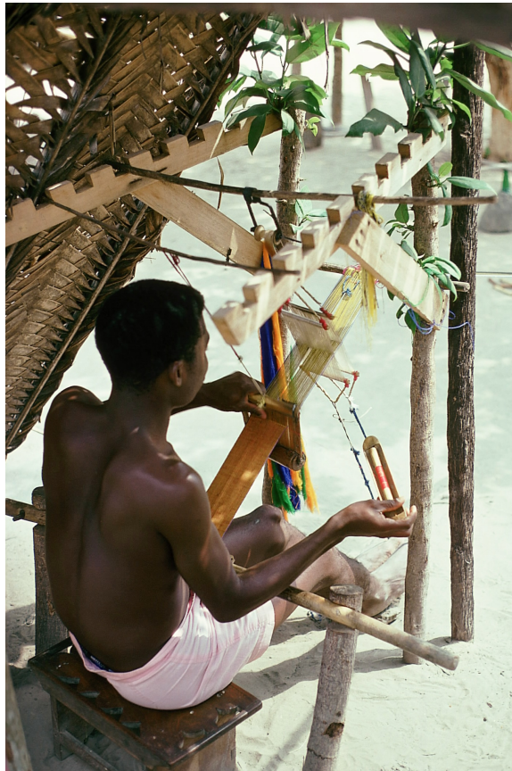
Figure 33. Weaver with left hand on beater and shuttle in right hand. Photograph by Gregory Bishopp.
