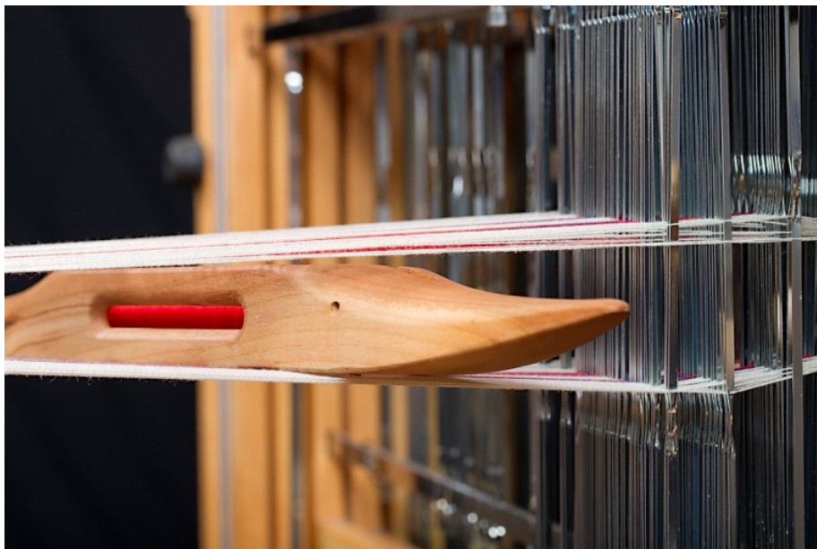
Figure 15. Shed allows shuttle holding weft thread (red) to pass through. Photograph by Tom Crosman.
