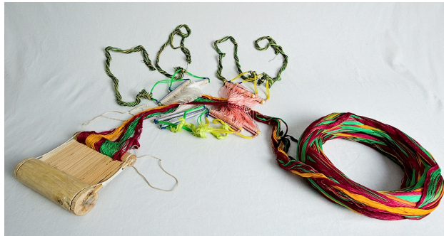
Figure 48. Strung beater, strung heddles, and crown ready to be placed on the loom. Photograph by Tom Crosman.
