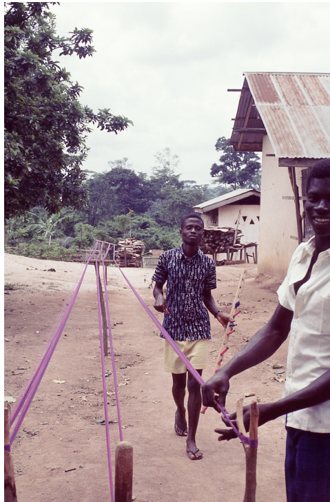
Figure 44. Measuring or laying of the warp. Warping specialist holding the bobbin carrier is measuring the warp threads. Photograph by Gregory Bishopp.
