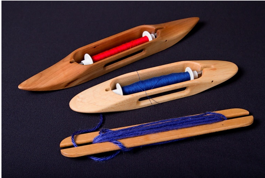
Figure 16. Shuttles of many styles and lengths. A stick shuttle in the foreground and boat shuttles with white bobbins holding weft in the background. Photograph by Tom Crosman.
