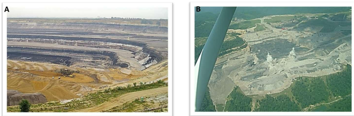
Figure 4.7: A) Strip mine for lignite coal at Garzweiler near Köln, Germany. Image from Wikimedia commons https://commons.wikimedia.org/wiki/File:Garzweiler.strip.mine.jpg B) Mountaintop removal in Eunice WV, photo by Roston, obtained from https://commons.wikimedia.org/wiki/File:Euniceblast3.JPG
